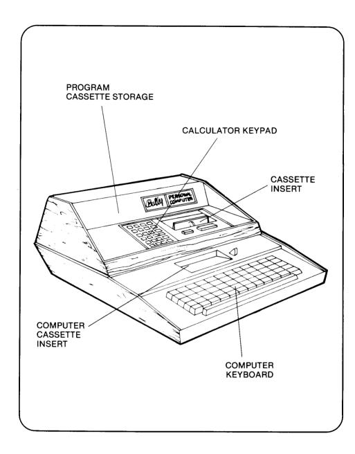
Shown above is the basic module of the personal computer connected to the add-on module. Not shown is either the digital or audio cassette decks which are separate accessories.
